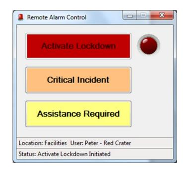
When a button is pushed the Remote Alarm Control reports the person and the location as an alarm in the Lenel Onguard Alarm Monitoring console and optionally as an email notification.
